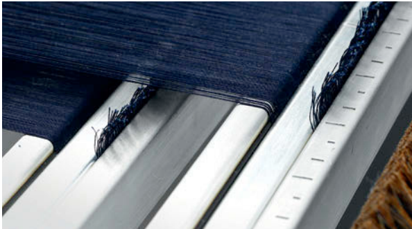
DETAIL VIEW: CLAMPED WARP
